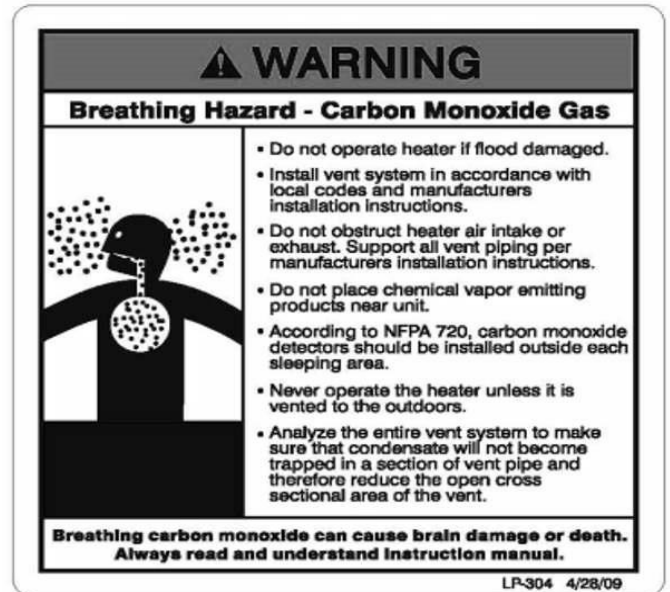
Figure 2 - CO Warning Label
