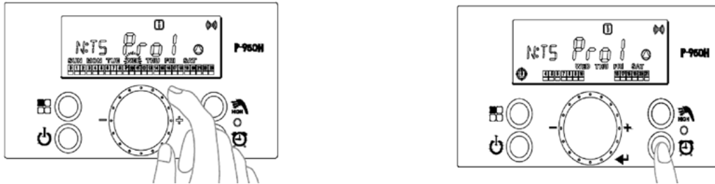
Figure 64 - A - Selecting the Day, Turning the Dial to Other Days, B - Setting the Time
