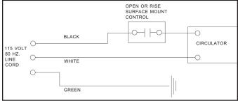
Figure 5 - Wiring the Control
