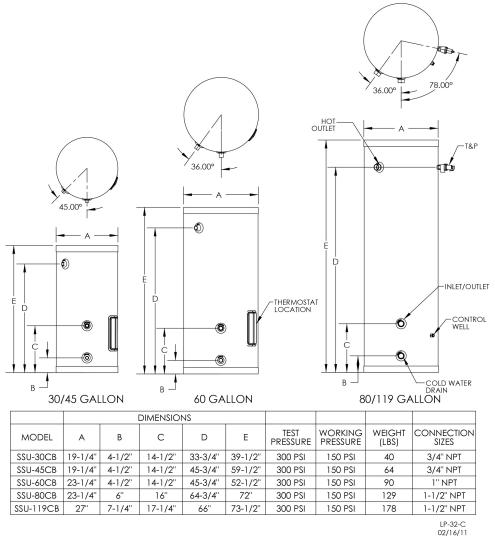
operation depending upon the type of **Figure 2 - Specifications and Dimensions** installation.) **60 Gallon S**
