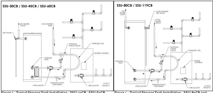
Figure 3 - Typical Storage Tank Installation - SSU-3oCB - SSU-6oCB Models
