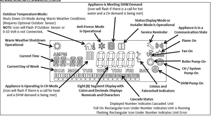
Figure 36 - LCD Display Detail
