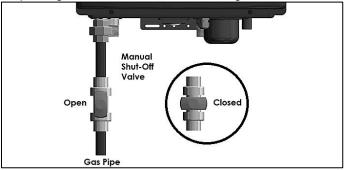
Figure 16 - Gas Line with Shut-Off Valve Detail
