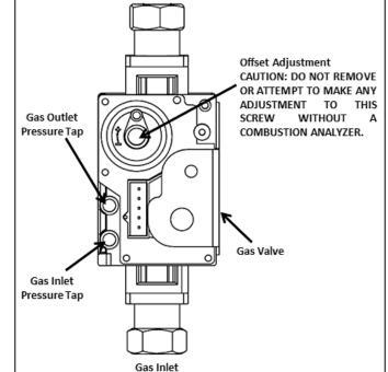
Figure 48 - Gas Valve Detail
