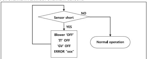
Figure 46 - DHW / OP / CH Overheat / Exhaust Overheat Sensors Error Analysis Tree
