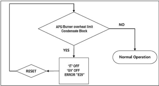
Figure 45 - APS / Burner Overheat Limit / Condensate Block Switch Error Analysis Tree
