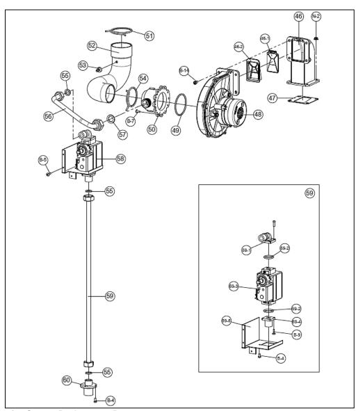
Figure 55 - Combustion System Replacement Parts
