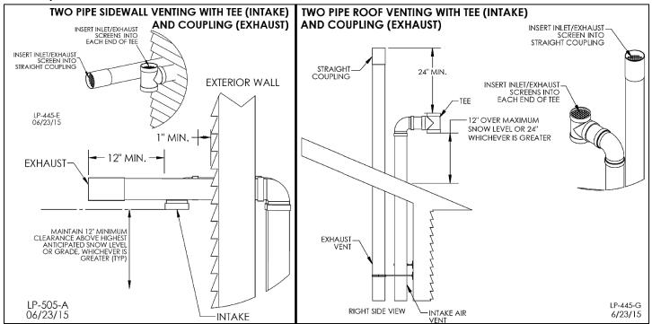
Figure 9 - Direct Vent, Roof and Sidewall Vent Terminations
