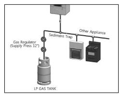
Figure 18 - LP Gas Piping Installation - NOTE: Capacity to be Not Less than Total Capacity of Connected Boilers
