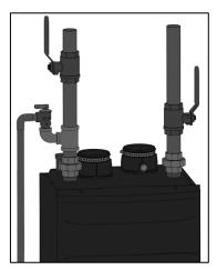
Figure 26 – Pressure Relief Valve
