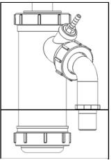
Figure 13 – Internal Condensate Trap
