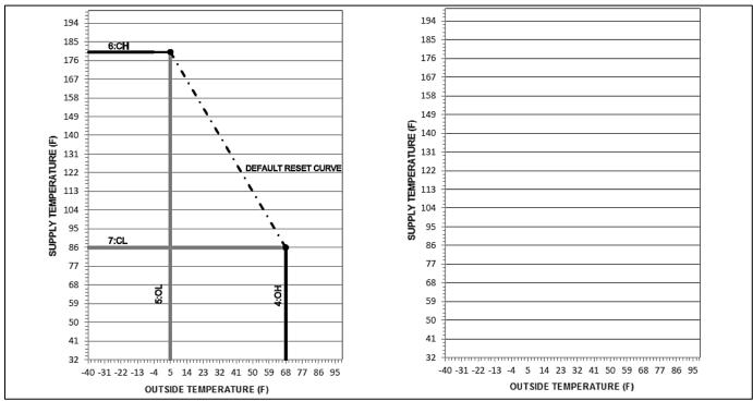
Figure 47 - Outdoor Reset Curve - See Installer Mode for Curve Setting Descriptions
