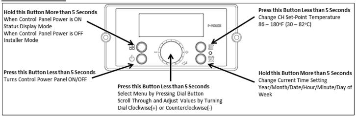
Figure 35 - Boiler Control Panel Detail
