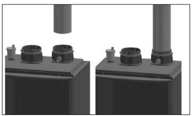
Figure 7 – Installing the 6" Length of CPVC into the Exhaust Vent Connection
