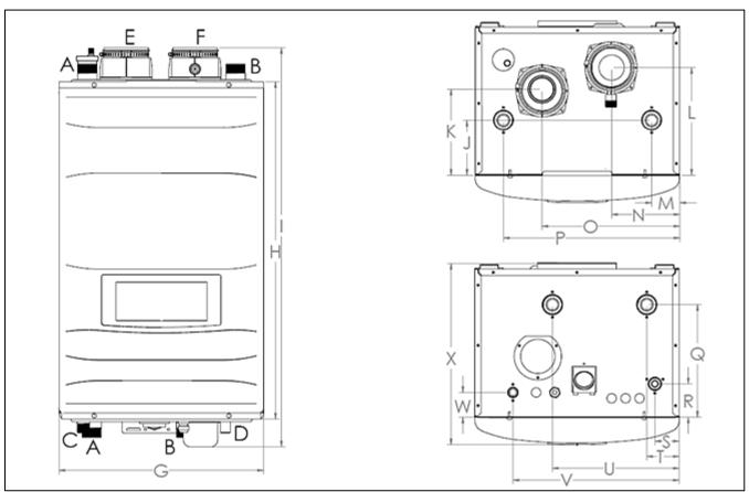
Figure 1 – UFT Specifications and Dimensions
