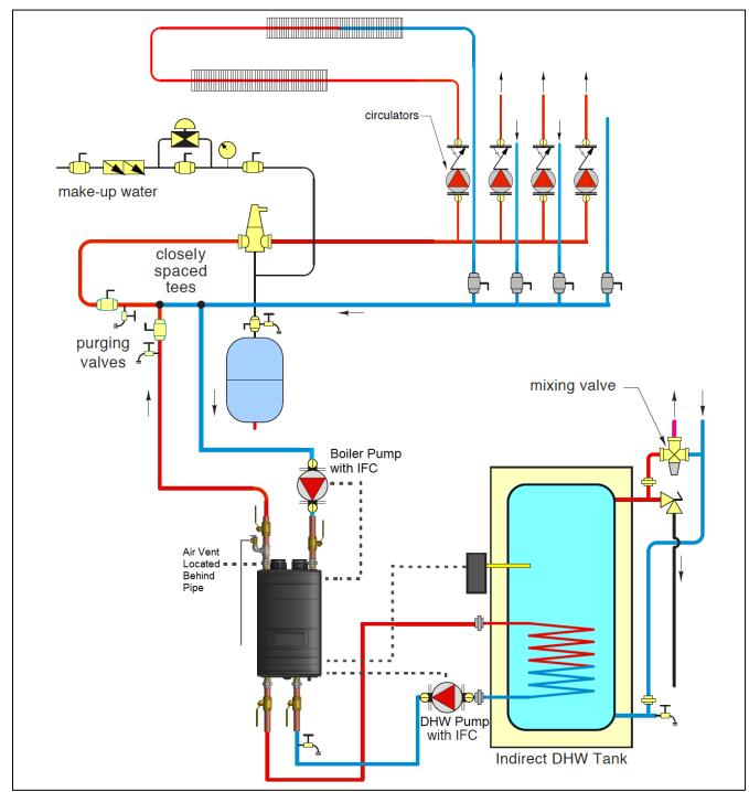
Figure 23 - Zoning with Pumps and Indirect Fired Water Heater - Primary/Secondary Shown
