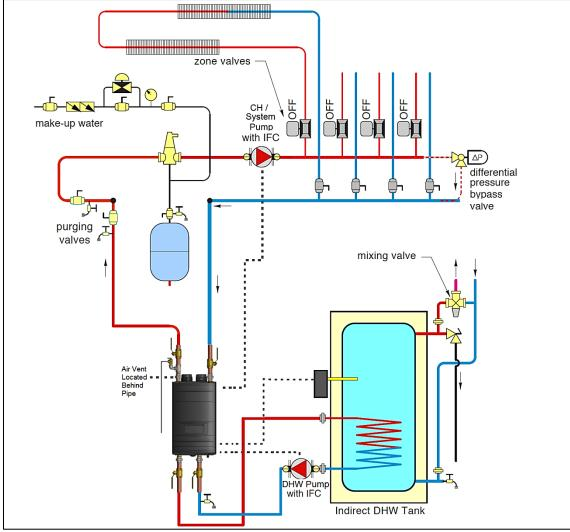
Figure 20 - Zoning with Zone Valves and Indirect Water Heating - Direct Piping
