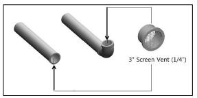
Figure 12 - Screen Installation
