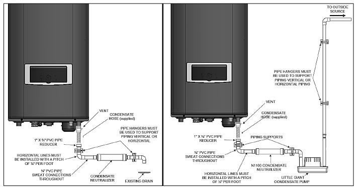
Figure 14 - Condensate Piping with Condensate Neutralizer / Condensate Piping with Condensate Neutralizer and Pump
