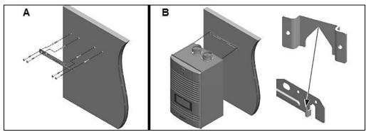
Figure 5 - Wall Mounting the Boiler
