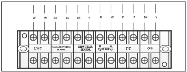
Figure 34 – Low Voltage Wiring Detail
