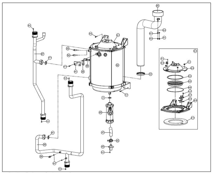
Figure 54 – Heat Exchanger Replacement Parts
