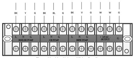
Figure 33 – Line Voltage Wiring Detail
